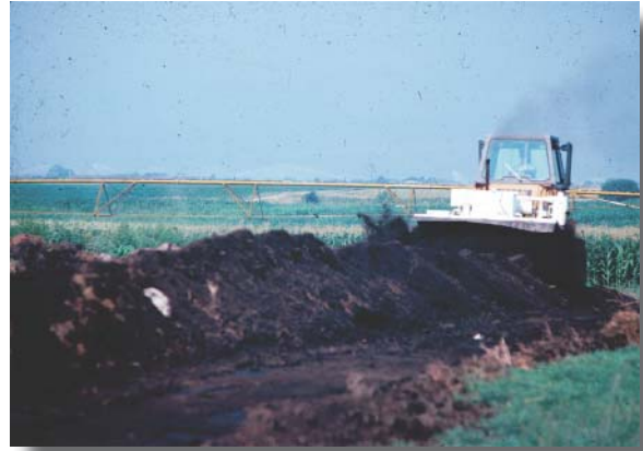
Field windrow turning of composted cattle manure with a Brown Bear auger turner.
